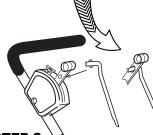
STEP 2: **Install Control Rod into** handle as shown above.
