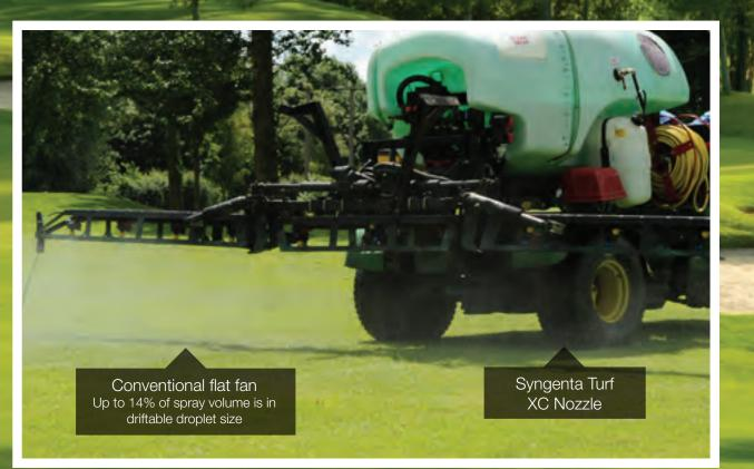
Syngenta XC Nozzles use innovative air induction technology – incorporating a cushion of air in every droplet – to reduce risk of drift and improve spray retention on the leaf.
