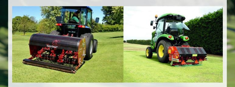
So why Verti Drain? It is useful to break up soil compaction from the years play, and it also provides desirable conditions for healthy root growth. By breaking up the compaction, it allows roots to penetrate more deeply into the soil and provides a conduit for surface water to reach the drains. This will allow for better absorbing of water and nutrients.
