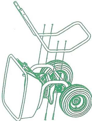
**3** Return the spreader to the upright position and attach the handle to the rest with four  $1\frac{1}{2}$ " carriage bolts and four lock nuts. **Be sure** that the main shutoff lever is facing up.
