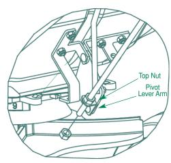
Pull the main shutoff lever to the closed position and look inside to see if the port holes are closed. If not, adjust the top nut down in small increments and check for closure. CAUTION - DO NOT ADJUST THE TOP NUT TOO FAR DOWN TO PREVENT BINDING THE MECHANISM. When the ports close completely, bring the bottom nut up and tighten both.
