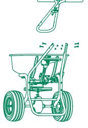
Place the bent end of the main shutoff connecting rod through the hole in the lever and secure it with a cotter pin on the right side.
