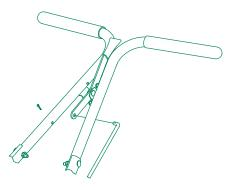
Thread one hex nut onto the lower end of the main shutoff control rod until it stops. Insert the rod through the pivot lever arm, as shown, and thread the second nut up to the pivot lever arm; do not tighten.
