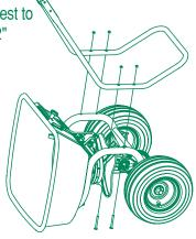
Return the spreader to the upright position and attach the handle to the rest with four 1 1/2" carriage bolts and four lock nuts. Be sure that the main shutoff lever is facing up.
