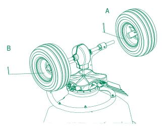
Place the spreader on its front side and attach the rest to the frame using four 2 1/2"
